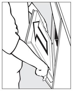
■ Hold the door securely at both sides, and lift it upwards off the retainers.
